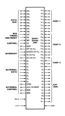
Figure 9. Z8591/Z8592 UPC Logic Functions
