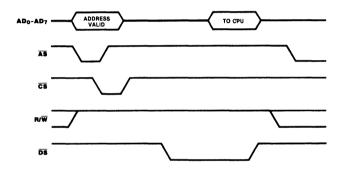
Figure 6. Z-BUS Read Cycle Timing
