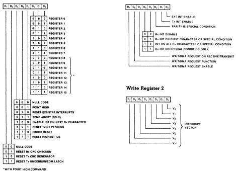
Figure 11. Write Register Bit Functions
