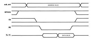
Figure 12. Read Cycle Timing
