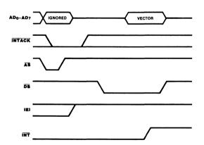
Figure 11. Z-BUS Interrupt Acknowledge Cycle
