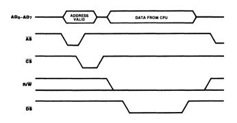
Figure 7. Z-BUS Write Cycle Timing
