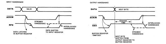
Figure 7. Interlocked and Strobed Handshakes
