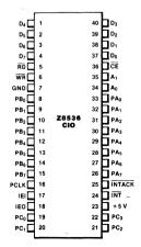
Figure 2. Pin Configurations
