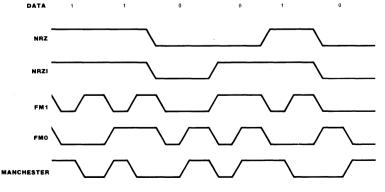
Figure 6. Data Encoding Methods
