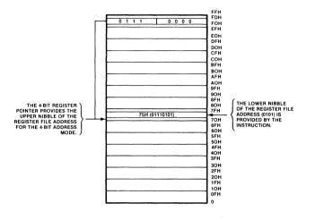
Figure 6. Register Pointer Mechanism
