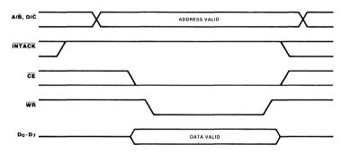
Figure 13. Write Cycle Timing
