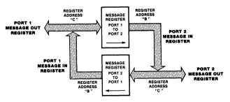
NOTE: Usable only for CPU/CPU interface. Figure 19. Message Register Operation
