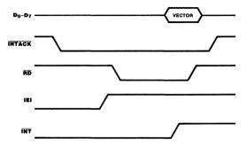
Figure 12. Non-Z-BUS Interrupt Acknowledge Cycle
