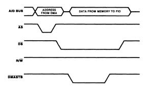
Figure 14. Z-BUS Memory to FIO Data Transaction
