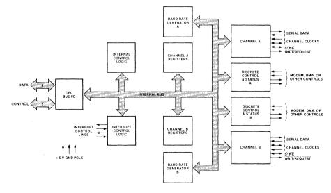
Figure 8. Block Diagram of SCC Architecture
