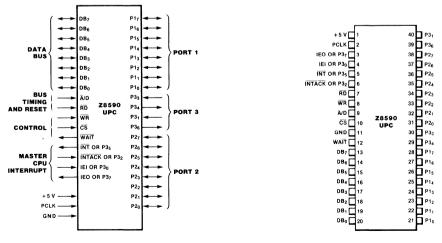
Figure 1. Z8590 UPC Logic Functions
