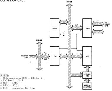
Figure 25. Typical Application: Node Controller
